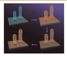
3D interconnected graphene/CNT networks are coated with porous carbon. The sp<sup>2</sup> graphene/CNT interlinked network gives the composites good electrical conductivity and a robust framework, while the meso-/microporous carbon and the interlamellar compartment between the opposite graphene accommodate sulfur and polysulfides, provide accessibility for liquid electrolyte to active materials, and restrain the shuttle phenomenon.
