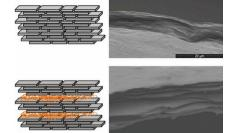
Graphene oxide-PMMA composite films with a multilayer laminate structure are shown to have greatly enhanced mechanical stiffness and strength compared to pure-graphene-oxide films. The thin polymer layers impart crack-deflection and stopping mechanisms that prevent catastrophic failure upon local failure and crack propagation, thereby making the material less sensitive to defects.
