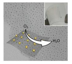
Reduced graphene oxide (rGO) films are decorated with non-overlapping Au nanoparticles using diblock copolymer micelles that provide controllability over the number density as well as the diameter of the nanoparticles. The rGO film enables the transferability of the Au nanoparticles without deterioration of their arrays, which exhibit high electrochemical activity in the oxygen reduction reaction.
