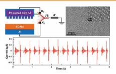
The two-electrodes-grounded triboelectric nanogenerator (TEG-TENG) is developed. The TEG-TENG can double the generated charges and enhance the output frequency compared to the traditional non-grounded TENG. The output energy at a load lower than 10  $M\Omega$  is also enhanced, and the enhanced ratio is more than 100 at a load of 100 k $\Omega$ .
