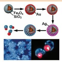
Highly asymmetric, interfaced dimers made of solid Au nanoparticles and hollow bimetallic nanoshells with different compositions are synthesized by combining the controlled growth of interfaced Au-Ag dimers and nanoscale galvanic replacement reactions on superparamagnetic colloidal substrates. The direct contact between the Au nanoparticle and the bimetallic nanoshells leads to possible strong couplings and novel properties.
